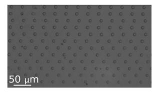
Figure 3. High-resolution e-jet printing of GOx dot array using a 5  $\mu$ m diameter nozzle at f = 20 Hz, v = 700  $\mu$ m/s.
