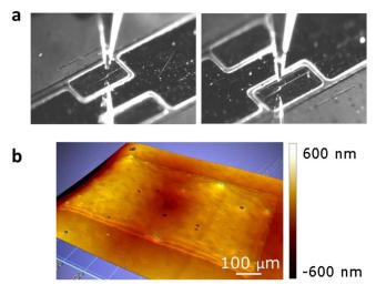
**Figure 5.** (a) E-jet printing of enzyme ink on Pt working electrodes of glucose sensor and (b) optical profilometry images of  $400 \times 800 \ \mu m^2$  (working electrode size) pad printed twice over the same area at  $f = 20 \ \text{Hz}$ ,  $v = 500 \ \mu m/s$ .
