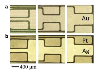
**Figure 2.** Optical microscopy images of (a) patterned Au on PI substrate prepared via microcontact printing, and (b) after Pt and Ag electrodes deposition by electroplating.
