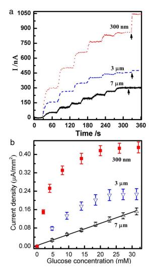
**Figure 6.** (a) Chronoamperometry of glucose sensor response to glucose concentration with printed GOx on Pt working electrodes and 300 nm, 3  $\mu$ m and 7  $\mu$ m thick outer PFSA membrane. Arrows indicate addition of 0.13 mM acetaminophen. (b) Current density vs. glucose concentration for these devices.
