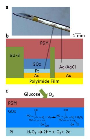
**Figure 1.** (a) The wrapping of the sensors around catheters with high radius of curvature  $\sim 250 \ \mu$ m, (b) schematic of a cross section of the amperometric glucose sensor on polyimide substrate and (c) schematic of the senors function and chemical reactions in the glucose oxidase (GOx) layer and on Pt working electrodes.
